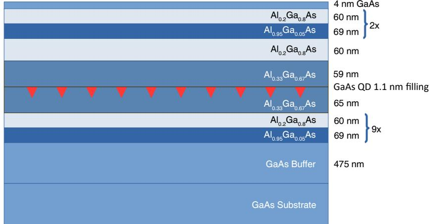
Figure 1: Structure of the sample used for temperature dependent entanglement measurements.
